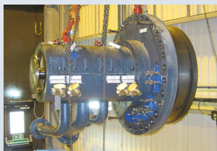
Compressor shaft prior to installation
