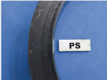
Contaminated seal face
