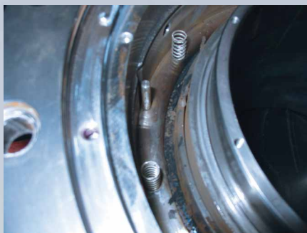
Contaminated seal area behind the stationary face
