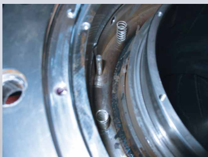
Destroyed seal faces after startup with contaminated sliding faces
