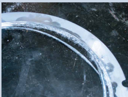
Contaminated dynamic sealing element
